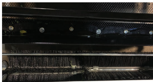
Rotating front brush, moves debris and filler into the hopper
