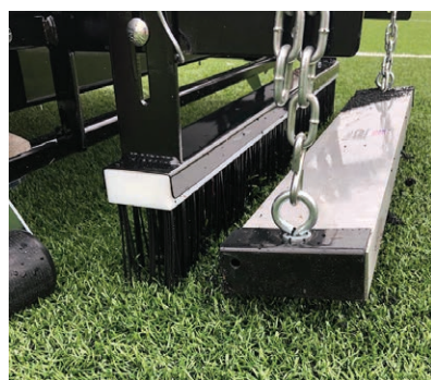
Optional rear mounted brush grooms turf and filler AND optional magnet collects hazardous debris such as pins, belt buckles, straps etc.
