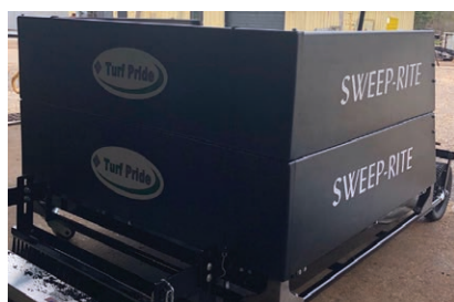
Optional stacking sides to increase hopper capacity for leaves and large debris
