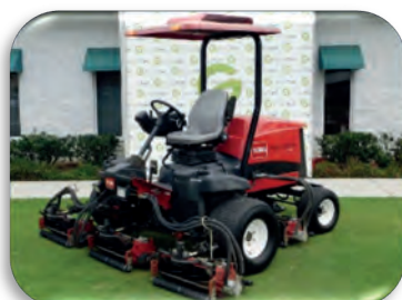
2015 Toro Reel Master 5510 4WD; 11 Blade DPA; Rear Roller Brushes; ROPS; Cool Top; Lights
