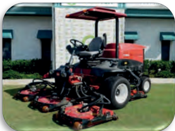
2016 Toro Grounds Master 4500D 4WD; 9ft cutting width; ROPS; Cool Top T4 2448 Hours
